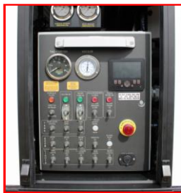
Air Excavation Controls
