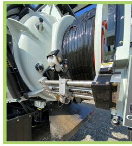
Tank Door, Hose Reel & Hose
