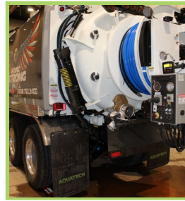
Tank Door, Hose Reel & Hose
